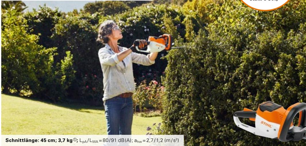
**Schnittlänge: 45 cm; 3,7 kg**
